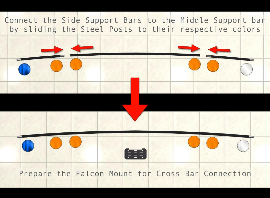
Secure Connections with Provided Allen Wrench Set and Screws Center the Falcon mount with the Curved Cross Bar. There are 2 Holes with Screws and Caps inserted in the Center of the Cross Bar to align with the Center of the Falcon Mount. Use those Screws and Caps to secure the Falcon Mount to the Cross Bar
