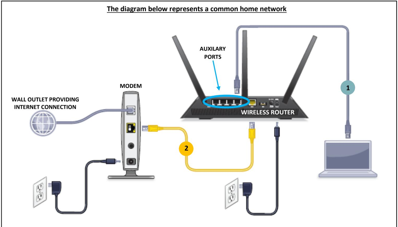
**Step 2.** The **BLUE CABLE (#1)** or any of the **AUXILIARY PORTS** on the **WIRELESS ROUTER** should be able to provide internet to your GCQuad. (see diagram above)
