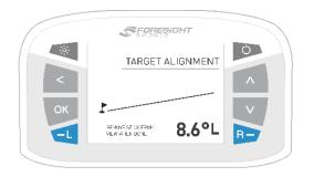
Alignment can be viewed and reset at any time from the Target Alignment menu in System Options. To reset alignment to factory default in this screen, press the OK key. Alignment is always reset when the unit is powered off.
