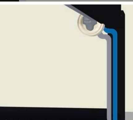
Continue to run the Cables down the Inside Face of the Right Side Support Beam, Securing with Cable Ties in various positions as needed
