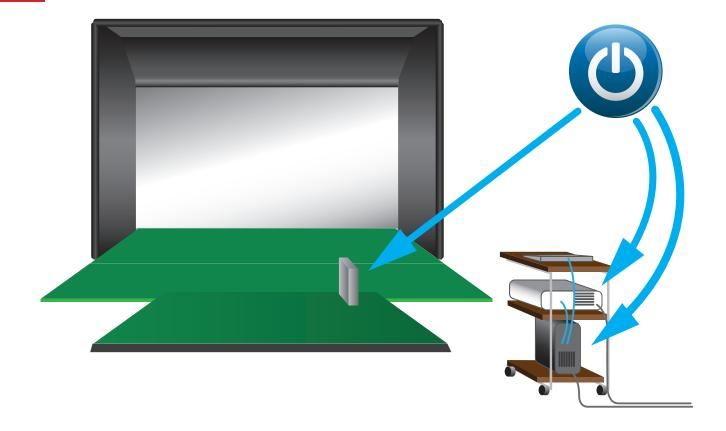
With the Projector on and projecting an image, move the Rolling Computer Cart toward the Hitting Screen until the image covers ALL FOUR CORNERS of the screen.
