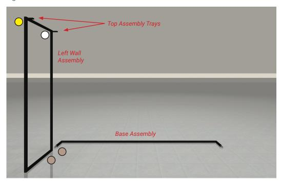
3B Connect the two assemblies as shown. Secure with 1 frame assemby screw.
